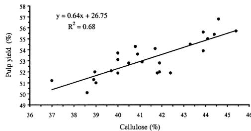
**Figure 2.** Relationship between cellulose content of cores at 0.9 m height and whole tree pulp yield at kappa 18 for 14 year old *E. nitens* [28].
