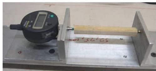
**Fig. 3** The fabricated device for measuring longitudinal dimensions in short samples
